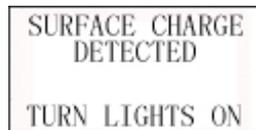
Turn lights on as prompted to eliminate battery surface charge, tester will then display the following messages in a sequence:
