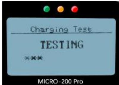
After the test finished, tester displays the effective charging volts, ripple test result and charging test result.
