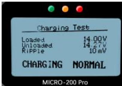
**NOTE:** If no increase rev detected, it shall be the fault of generator regulator or connection with battery failed. Tester will try 3 times to further detect, if still failed, it will skip the increase rev detect and the test result displays "No Volt Output".
