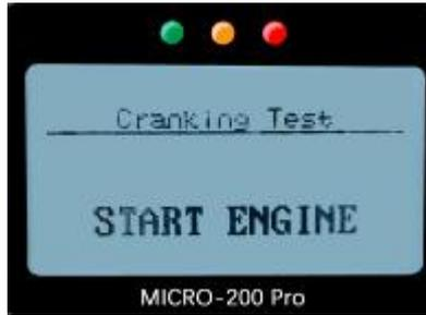
Starting the engine as prompted, tester will automatically complete the cranking test and display the result.
