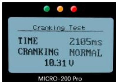
When cranking test is abnormal, battery test result will also be displayed at the same time.
