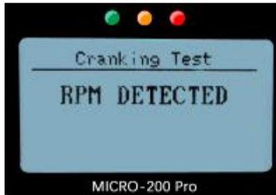
Normally, cranking voltage value lower than 9.6V is regarded as abnormal and it is OK if it is higher than 9.6V.
