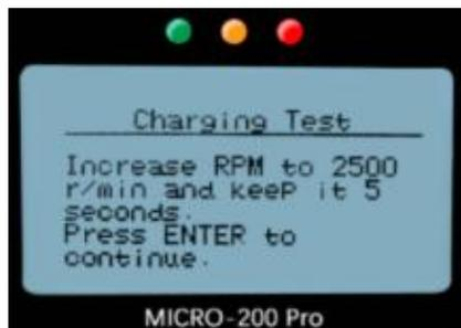
Tester starts the charging volt test after increase rev detected.
