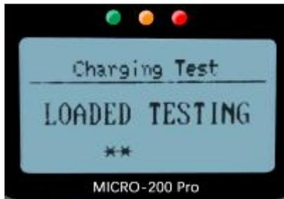
**Note: Do not shut down the engine during the test. All electrical appliance and device are in OFF state. Turn on/off any electrical appliance in the vehicle during the test will affect the accuracy of the test result.**
