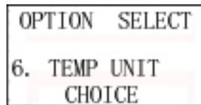
Firstly, press OK key one time, then use UP/DOWN arrow to choose °C or °F. After successful setup, it shows "OK" for 2 seconds, then return to the previous interface.
