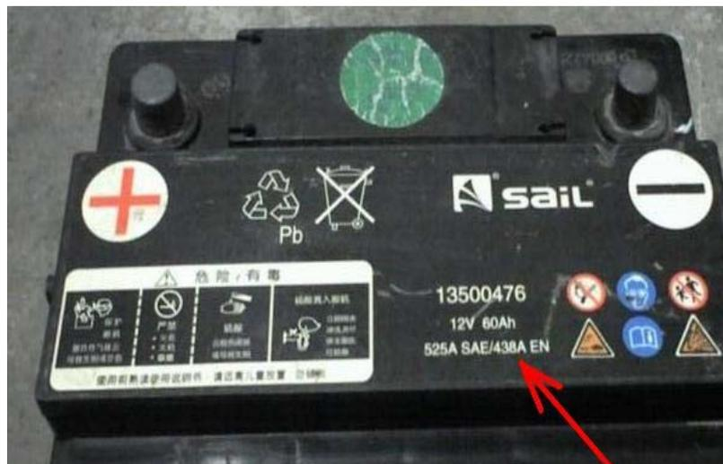
**CCA:** Cold Cranking Amps, specified by SAE&BCI, most frequently used value for starting battery at 0°F (-18°C)
