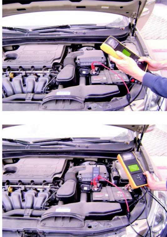
As the minimum width of the current clamp jaw is only 28mm, choose the connection cable or connection pole with diameter less than 28mm to test. Otherwise, the current clamp jaw cannot close completely.
