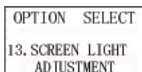
This function is to adjust the screen backlight brightness for power saving mode and for clear view of the displayed characters under the sunlight.
