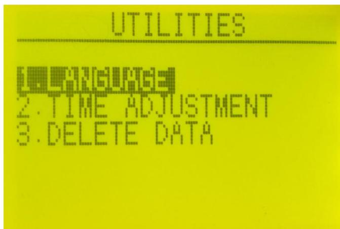
3.8.1 Select "TIME ADJUSTMENT" and press "OK" to enter the time setting
