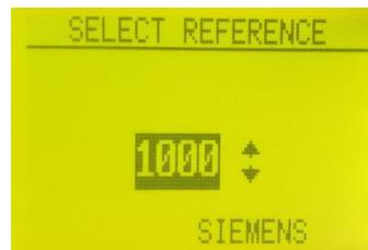
Press the up and down key to adjust the value of the standard values, press "OK" to confirm the standard value input and return to the boot main interface.
