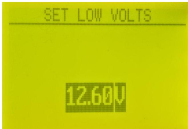
12V voltage default low voltage reminder for 12.60V, you can press up and down keys to adjust the reminder voltage value.
