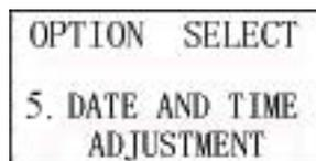
Adjustment is in the sequence of Year, Month, Date, Hour, Minute. This adjustment sequence does not affect the date and time format.
